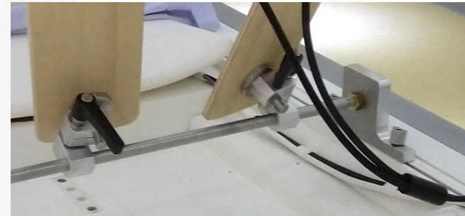
With the clamping lever it is easily to lose or fixate the wooden slabs
